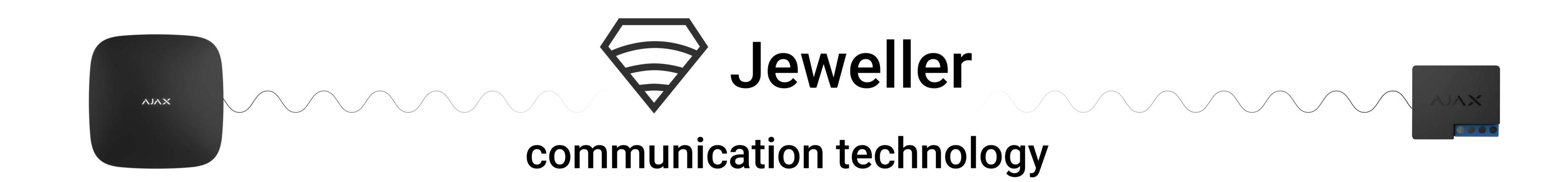
**Jeweller** is a **wireless data transfer protocol** to provide fast and reliable two-way communication between the hub and connected devices. The protocol helps monitor and control connected devices via Ajax apps. All data transfers — from the hub to a device or the cloud — are delivered in small data packets and protected with floating key encryption.
