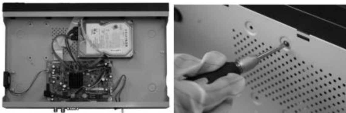
Figure 4.3 Placing the HDD and Fastening the Screws
