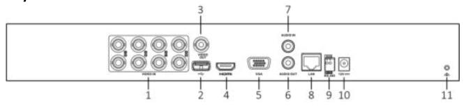
\*: The rear panel of iDS-7204HUHI-M2/S and iDS-7216HUHI-M2/S provide 4 or 16 video input interfaces.
