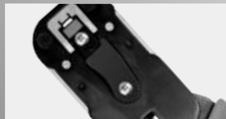
SLIDING TOOL LOCK to keep the crimp tool closed when not in use
